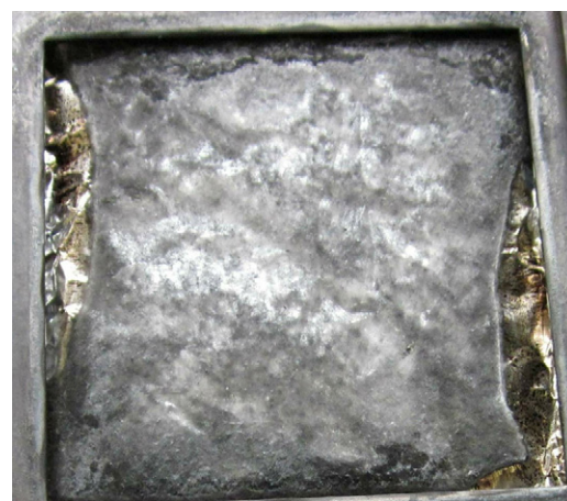
Fig. 2. UCF sample after cone calorimeter testing at 10 kW/m 2 flux.
