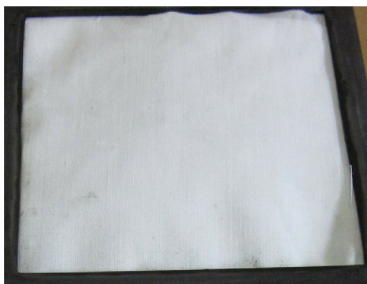
Fig. 3. BCF sample in sample holder before testing on cone calorimeter.
